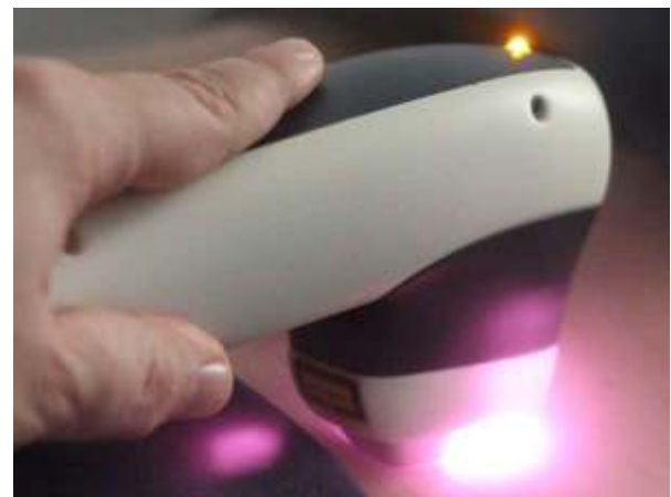
The epilation handpiece of the Asclepion MeDioStar NeXT laser with integrated Peltier cooling element
